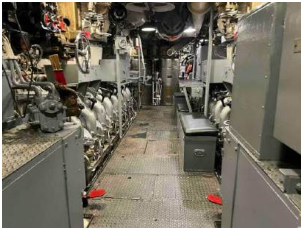
One of two diesel generator rooms, each with two diesel generators.
