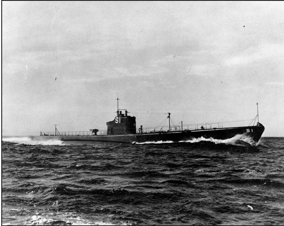
❖ **Armament: 8 × 21” torpedo tubes (four forward, four aft), 24 torpedoes, 1 × 3”/50 caliber deck gun, four machine guns.**
