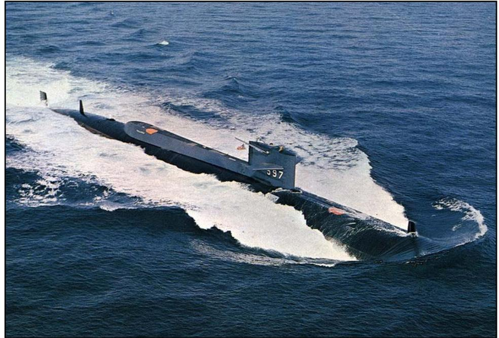
❖ She was built to test the new bow sonar and amidships torpedo room configuration that is now standard for US submarines.
