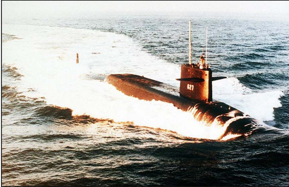
❖ The James Madison class of 10 submarines were an evolutionary development from the Lafayette class of fleet ballistic missile submarine. They were identical to the Lafayettes except for being designed to carry the Polaris A-3 missile instead of the earlier A-2.
