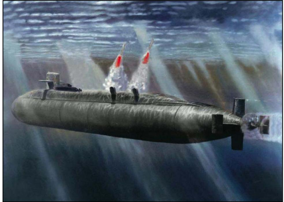
❖ 22 of the 24 Trident missile tubes were modified to contain large vertical launch systems (VLS), one configuration of which may be a cluster of seven Tomahawk cruise missiles. In this configuration, the number of cruise missiles carried could be a maximum of 154.
