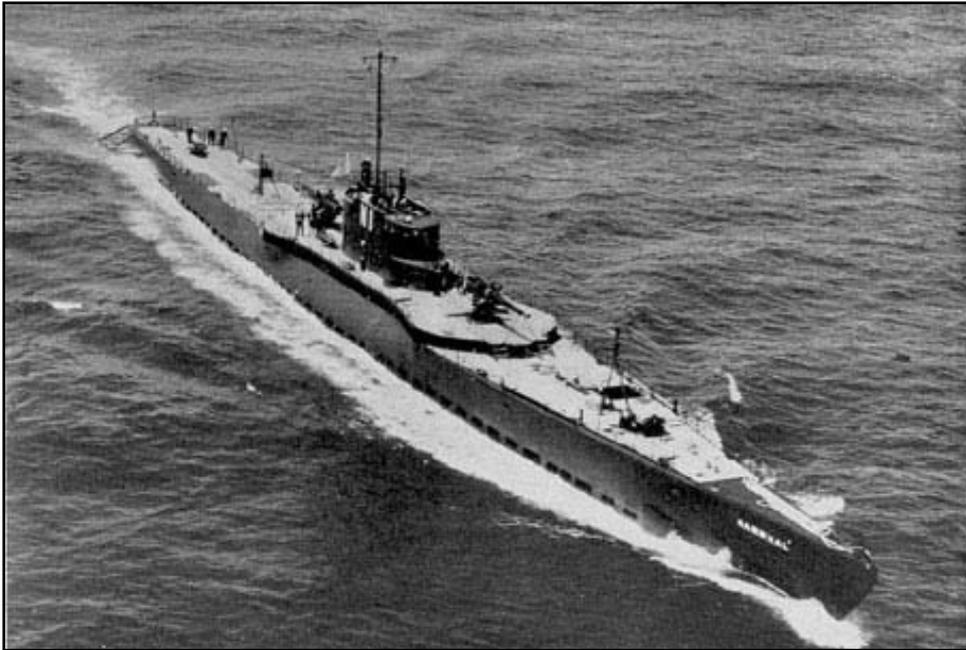
❖ Originally, a small scouting seaplane was to be carried in a water-tight hangar abaft the conning tower.
