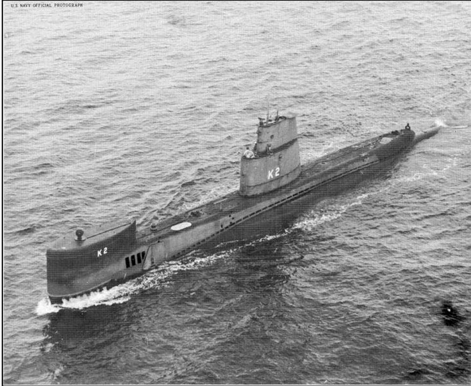
❖ The three SSK boats, Barracuda (SSK-1), Bass (SSK-2), and Bonita (SSK-3), were built around the large BQR-4 bow-mounted sonar array as part of Project Kayo, which experimented the use of passive acoustics with low-frequency, bow sonar arrays.
