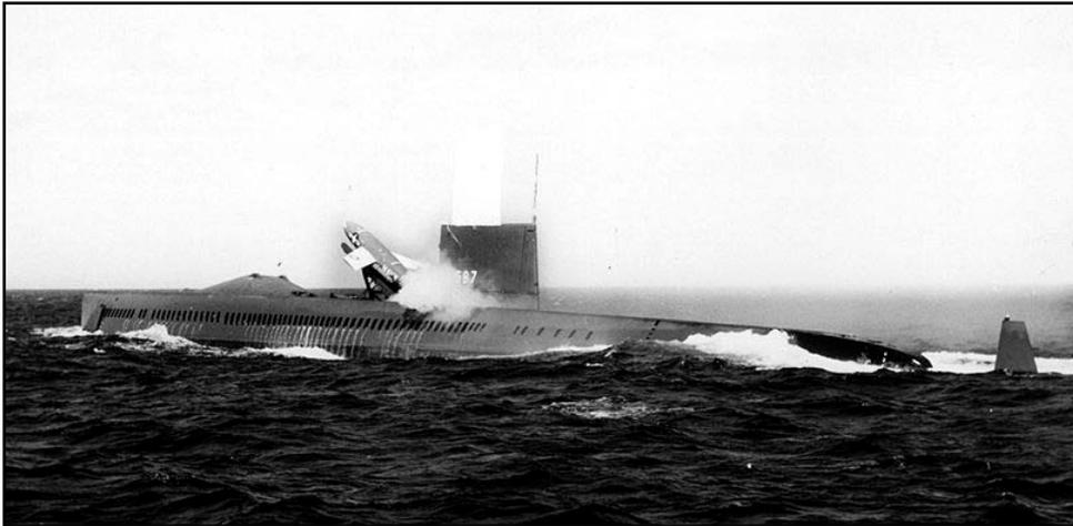
❖ Begun as a diesel-electric submarine but completed with nuclear power, Halibut was the first submarine designed to launch guided missiles.
